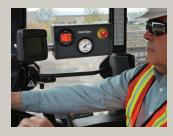
Host vehicle control box provides loader operator with a comprehensive engine monitoring computer, tachometer and hard-wired emergency stop (E-Stop).
