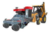
Front wheel assist enables the AZ-500B to be operated on smaller host vehicles by offsetting a portion of the machine's weight to a front wheel system. Includes remote-controlled power steering.
