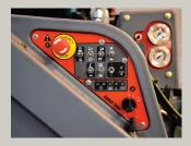
**Side-mounted machine control panel** gives groundsman safe and easy control of all machine functions and emergency stop (E-Stop).
