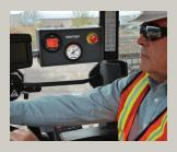
Host vehicle control box provides loader operator with a comprehensive engine monitoring computer, tachometer and hardwired emergency stop (E-Stop).
