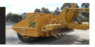
The Auto Control System for grader mounted rollers maintains constant compaction force to the roller over varying terrain and surfaces.
